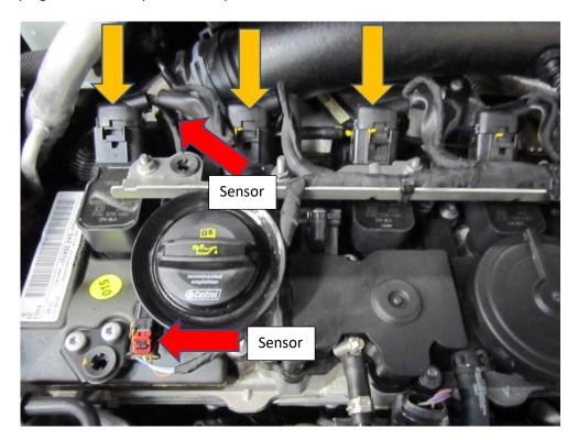
10. First locate the second coil pack from the left of the engine when standing in front of the car. Now move the loom rail to gain access to the coil pack retaining nut. Using a 10mm ratchet/spanner undo this nut and remove it from the coil pack. The coil pack should now lift out - you may need to use a flat blade screw driver or trim tool to help persuade it out.
