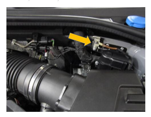
5. Now place the catch can bracket over the screw poles in front of the earth bracket and slide the cables back into place then tighten up the 10mm & 13mm nuts.
