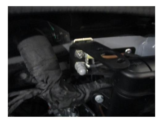
6. Attach the catch can to the bracket by mounting the catch can underneath the bracket and screw into place using the 4mm cap head screws provided. There is adjustment in the bracket to allow you to change the angle of the catch can.
