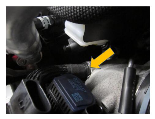
13. Using the longer hose from the catch can kit push fit the rounded end breather pipe adaptor. You will hear a click which tells you it is located properly. This will now push fit onto the turbo elbow.
